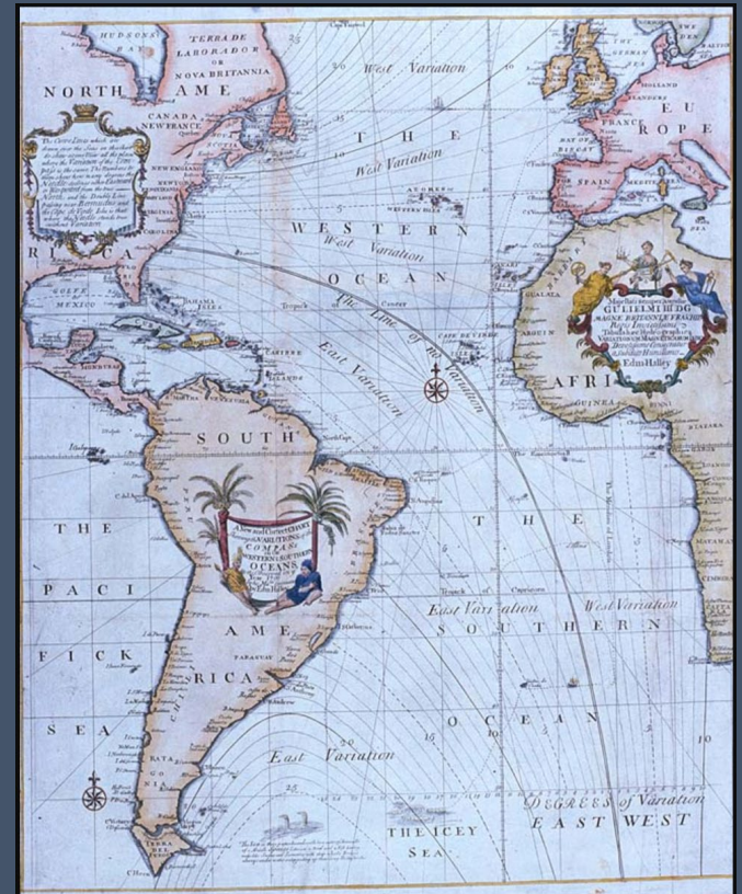
Edmond Halley's New and Correct Chart Shewing the Variations of the Compass (1701), the first chart to show lines of equal magnetic variation. Wikimedia.org
